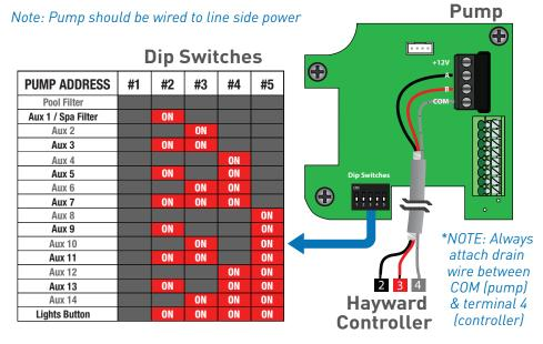
2b. Set all pump DIP switches to the down/off position
